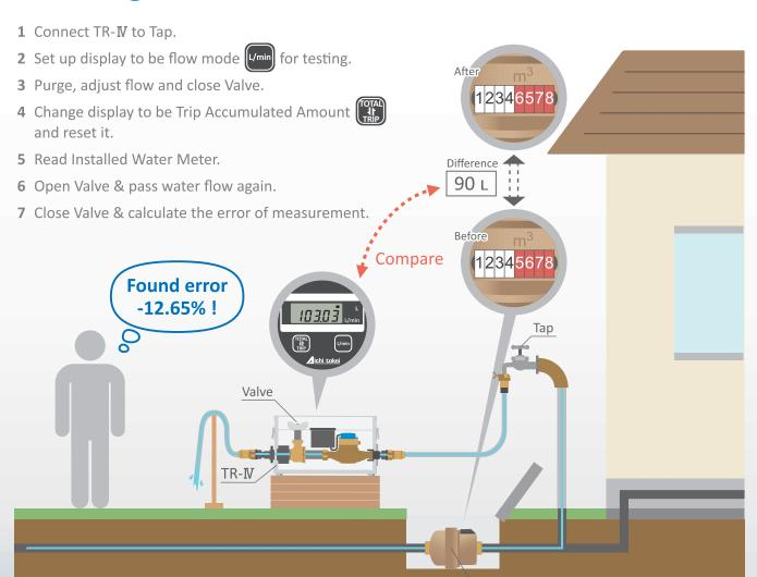
**TR-IV**Portable Water Meter Test Kit
